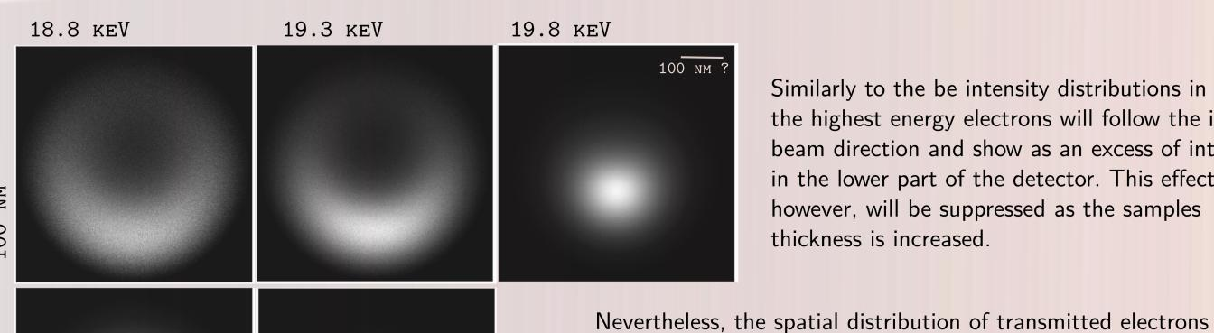
Similarly to the be intensity distributions in EBSD, the highest energy electrons will follow the incident beam direction and show as an excess of intensity in the lower part of the detector. This effect, however, will be suppressed as the samples thickness is increased.
