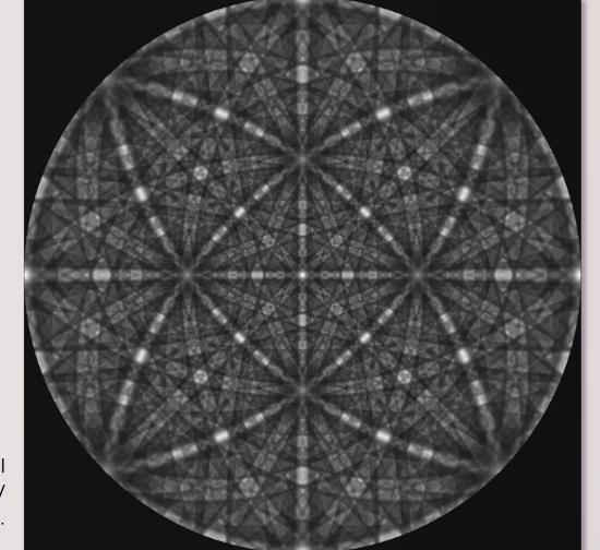
If the probabilities are calculated for all independent scattering directions a 'master TKD pattern' is obtained from which any needed TKD patterns can be extracted via bi-linear interpolation. This method reduces the number of calculations needed for a specific set of patterns as the multibeam dynamic simulations must only be carried once for all beam directions.
