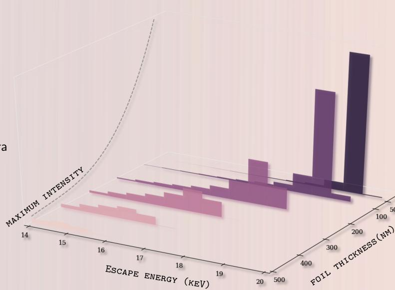
over a narrow range of energies. The inverted intensity distribution for the 100 nm film 18.8 keV bin is due to the fact that the film thickness is comparable to the mean free path. While equation (1) is independent on the diffraction
