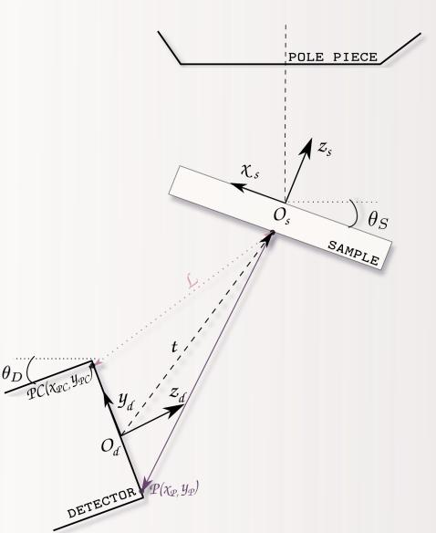
TKD Geometry where PC is denotes the pattern center and L is the distance between the detector
