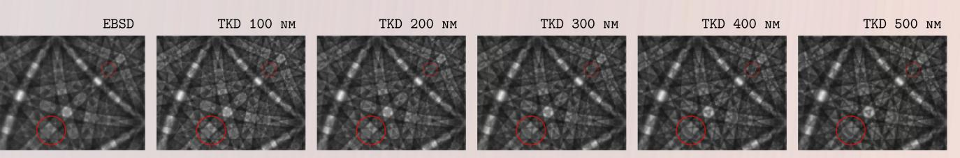
Same area on the Master Pattern comparison between EBSD and TKD for various sample thicknesses. TKD patterns show much finer diffraction details which are very dependent on the sample thickness. The large circle fallows the behaviour of a dark gray feature which vanishes for very thin samples. The smaller circles follow the gain of contrast of a set of higher order Kikuchi lines as the sample thickness is increased.
