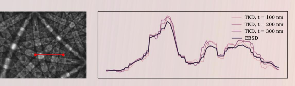
Intensity line scan (red line on left) comparison between EBSD and TKD patterns simulated for Ni in same sample geometry. The TKD patterns not only show higher contrast features (defined as the difference between maximum and minimum intensity), but also finer details than the EBSD one.
