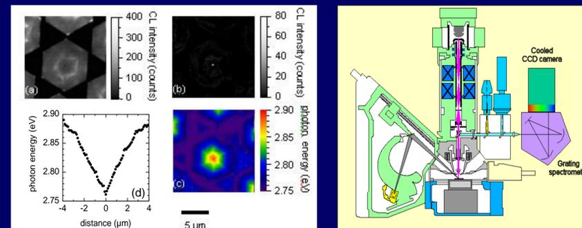
CL spectral imaging. (a) and (c) show the peak intensity and energy respectively of the QW emission from the facets, whilst (b) shows the intensity of the 2.37 eV apex-related band. The linescan (d), showing the QW peak energy varying across the pyramid, was extracted from a horizontal line through the apex in (c).
