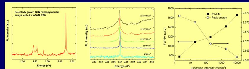
PL spectrum of single micropyramid containing 5 quantum wells
