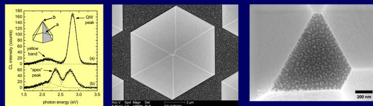
Room temperature CL spectra showing the emission from (a) a facet center and (b) the apex.
