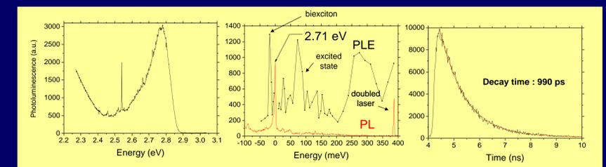
One-photon excitation, showing QD emission superimposed with a background originating from the QW emission.
