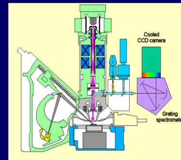
Strathclyde's modified CAMECA SX100 electron microprobe and CL spectrum mapping facility
