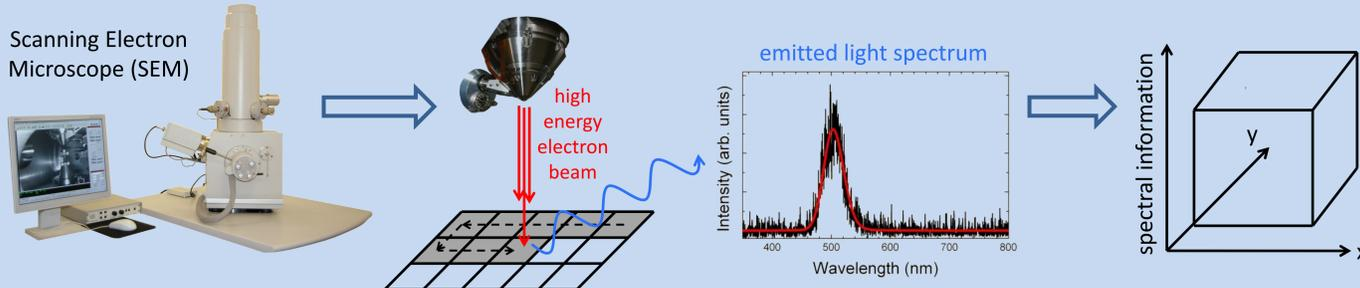
A Scanning Electron Microscope is used to investigate nanoscale features on the sample surfaces. In order to examine the light emitted from the sample, the electron beam is scanned across the surface while simultaneously acquiring a cathodoluminescence (CL) spectrum at each point on the sample. The result is a large 3D data set, or hyperspectral image, which can be treated mathematically to extract important patterns of behaviour.
