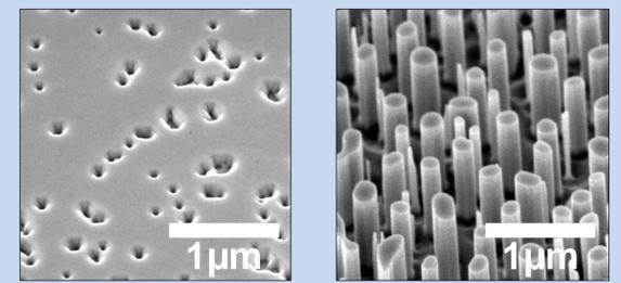
Before etching      After etching
