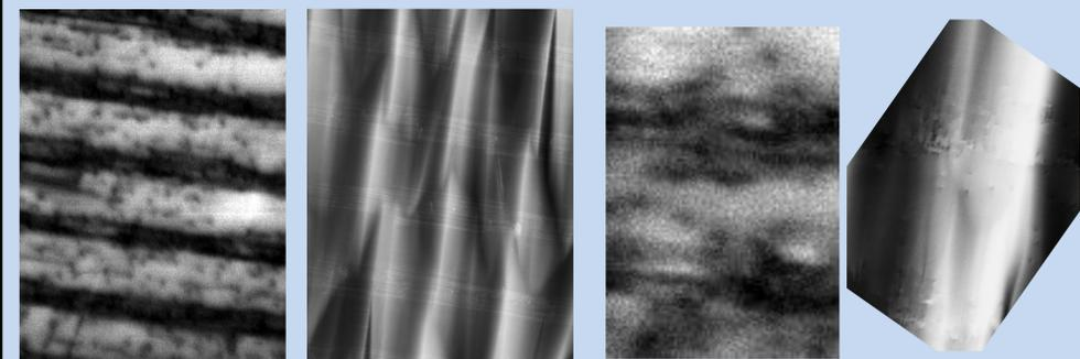
ECCI reveals the presence of dislocations and stacking faults in our samples. The CL reveals that these defects result in a reduction in luminescence intensity.
