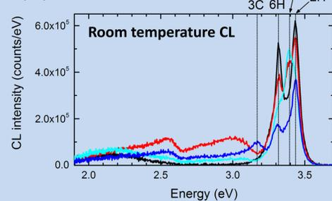
The observation of a number of peaks ranging from 3.2 eV to 3.45 eV indicates the presence of polytypes in our semi-polar GaN samples.
